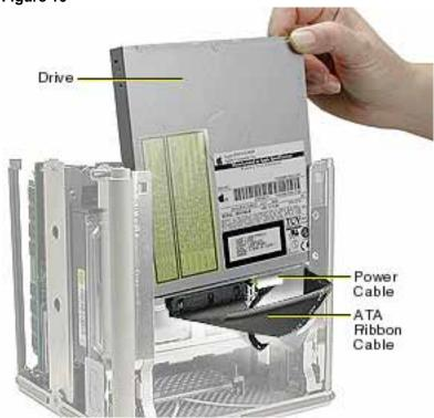
5. Slide the optical drive up and out of the chassis.
